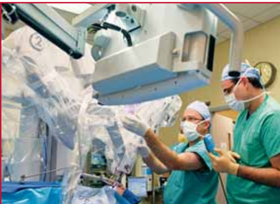
Drs. David Kutler (left) and Marc Cohen position the robotic arms to provide access to difficult-to-reach areas of the throat.
